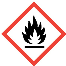
Substance marking "Flammable"
