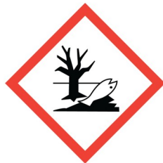
Substance marking "Hazardous to water"
